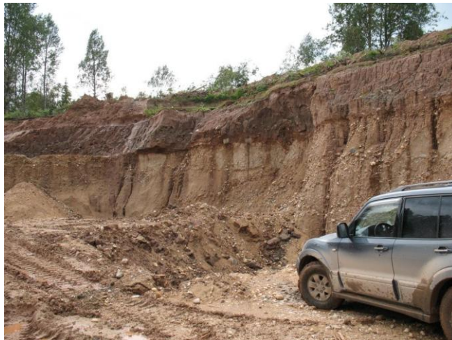
Picture 3. Good stony material for road pavement under a two-meter layer of clay. Tikhvin region, Russia
